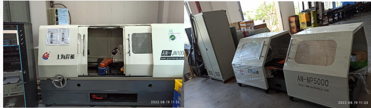
Just upgraded CN dynamic fatigue testing machine -5000Nm~5000Nm 0-45° angle 1-4Hz
